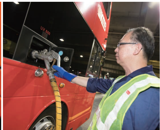
The aircraft-style "Posilock" fuel filling system is used to prevent spillage 採用飛機使用的「Posilock」加油系統，防止燃油外溢
